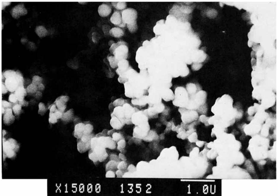
Fig. 9. PVC primary particles at very low conversion ( \times 15,000 ) (run 9, conversion below 1%).
